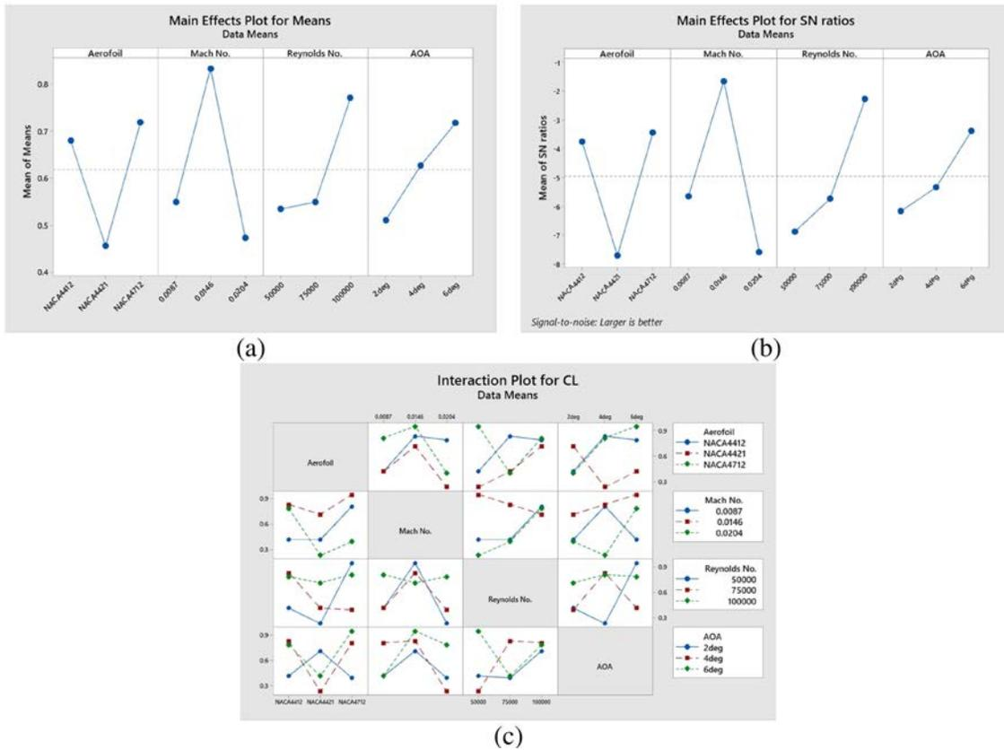
**Figure 9:** (a) Effect of Aerofoil, Re, M and AOA on mean  $C_L$ , (b) Signal to Noise effect plot for  $C_L$  and (c) Plot for interaction of aerofoil, M, Re and AOA.
