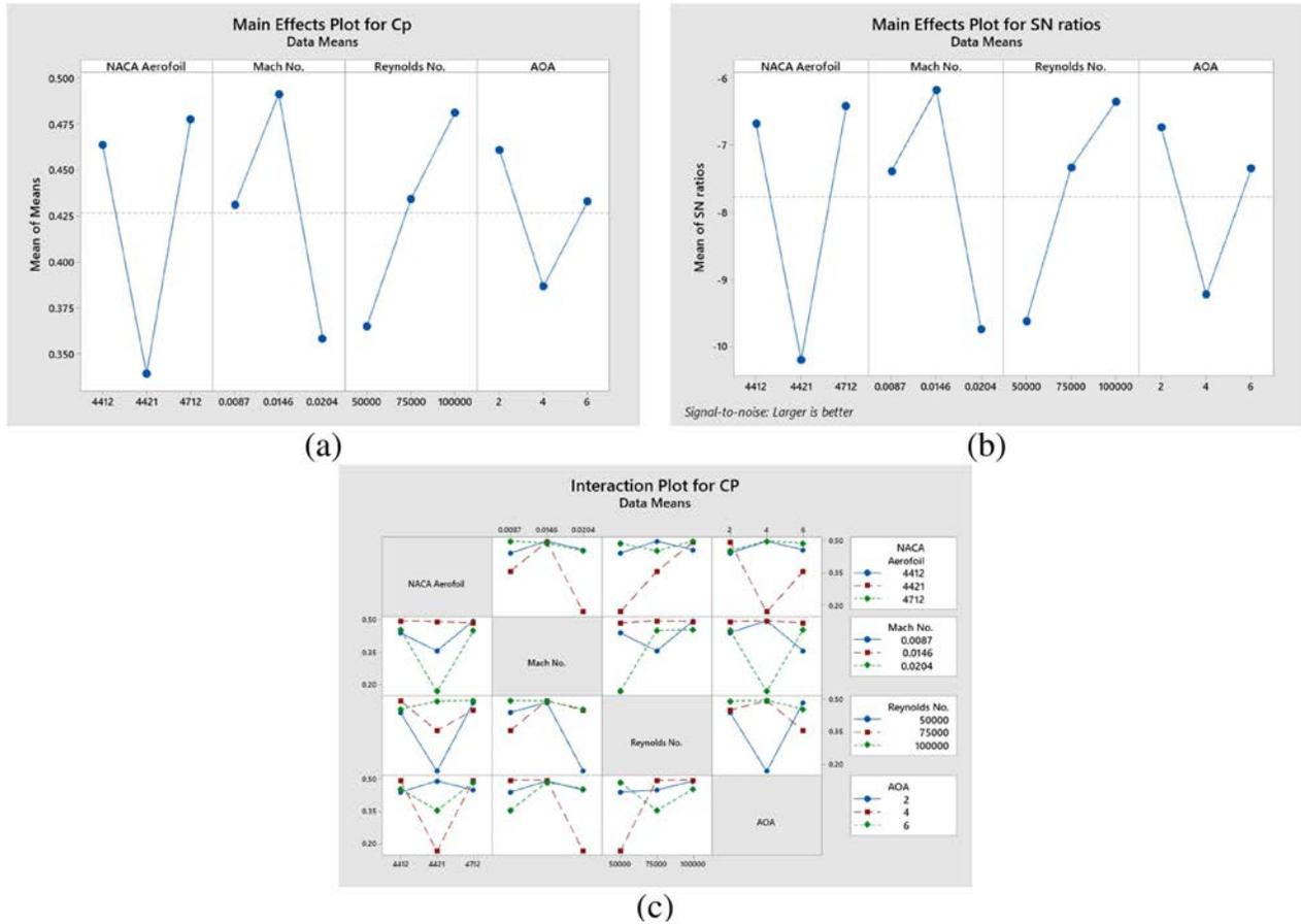
Figure 11: (a) Effect of Aerofoil, Re, M and AOA on mean  $C_P$  (b) Signal/Noise ratio effect plot and (c) Plot for aerofoil, M, Re and AOA interaction.
