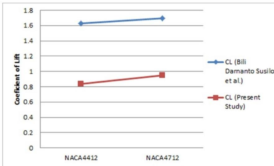
Figure 8: Comparison of lift coefficients of NACA4412 and NACA4712.
