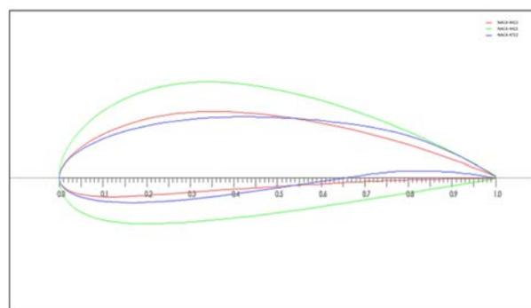
**Figure 4:** NACA 4412, 4421 and 4712 aerofoil profiles.
