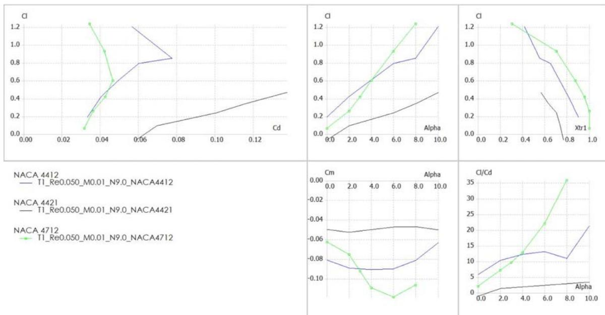
**Figure 5:** Plots between various parameters at Mach 0.0087 and Re 50000 for NACA4412, 4421 and 4712 using Q-blade software.
