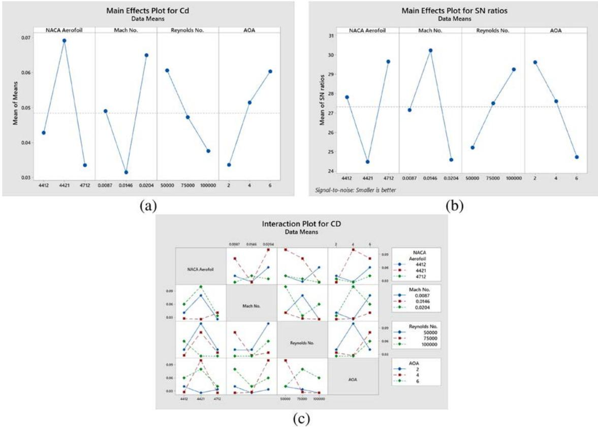
Figure 10: (a) Effect of Aerofoil, Re, M and AOA on mean  $C_D$ , (b) Signal to Noise effect plot for  $C_D$  and (c) Plot for interaction of aerofoil, M, Re and AOA.
