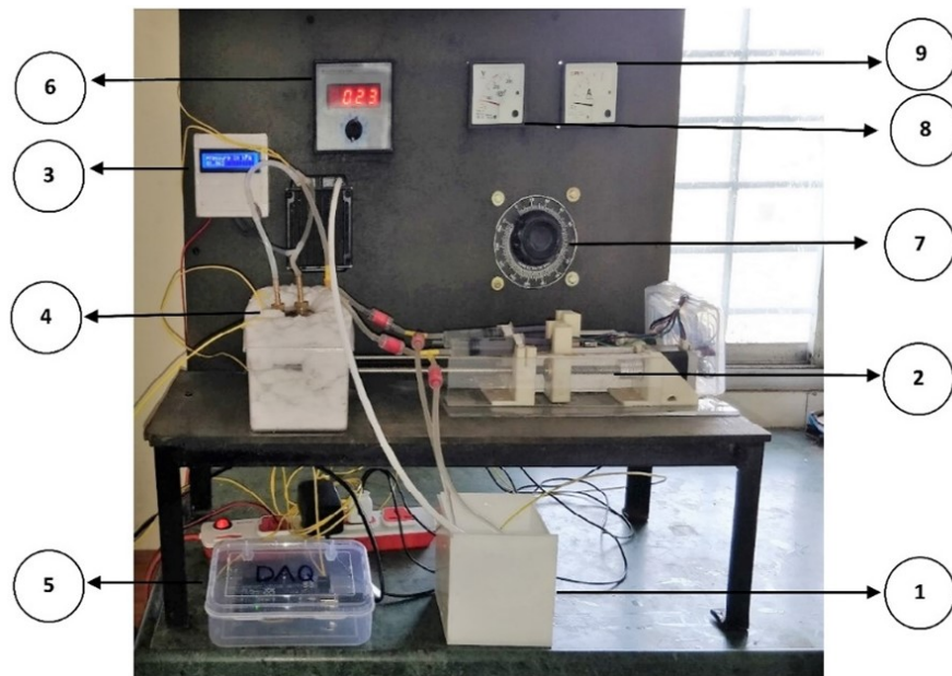
Figure 2: Typical experimental setup where Coolant tank (1), Syringe pump (2), Digital differential pressure transducer (3), Microchannel test section (4), Rectangular cartridge heaters (5), Thermostat (6), Data Acquisition system (7), Computer (8), Radiator (9), Digital temperature indicator (10) and Glass wool.
